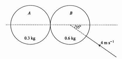
A smooth sphere A, of mass 0.3 kg, is at rest on a horizontal surface. A second smooth sphere B, of mass 0.6 kg and with the same radius as A, is moving on the surface and collides with A. Immediately before the collision, the velocity of B is  $4 \,\mathrm{m \, s^{-1}}$  at an angle of  $35^\circ$  to the line of centres (see diagram). The coefficient of restitution is 1. Find the speed and the direction of motion of B immediately after the collision.
